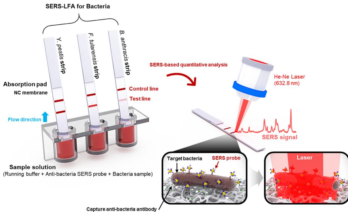
**Fig. 2.** Operating principle of the SERS-based LFA sensing platform. LFA strips for *Y. pestis*, *F. tularensis*, and *B. anthracis* were dipped into wells of a 96-well ELISA plate containing mixtures of SERS nanotags and different concentrations of bacteria in buffer solution. The immunocomplexes that formed migrated by capillary action toward to the test line, where their Raman signals were measured and analyzed.
