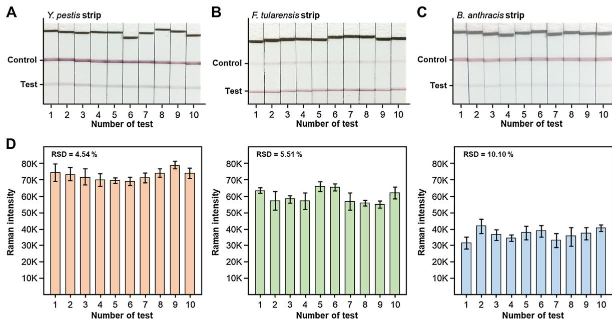
**Fig. 4.** Reproducibility test of SERS-based LFA strips. Digital photographic images of 10 strips for (A) *Y. pestis*, (B) *F. tularensis*, and (C) *B. anthracis*. Test concentration was  $10^7$  CFU/mL for all three bacteria. (D) Variations in corresponding Raman peak intensities at  $1616\text{ cm}^{-1}$  for three bacteria. Error bars indicate the standard deviations of five measurements for each strip.
