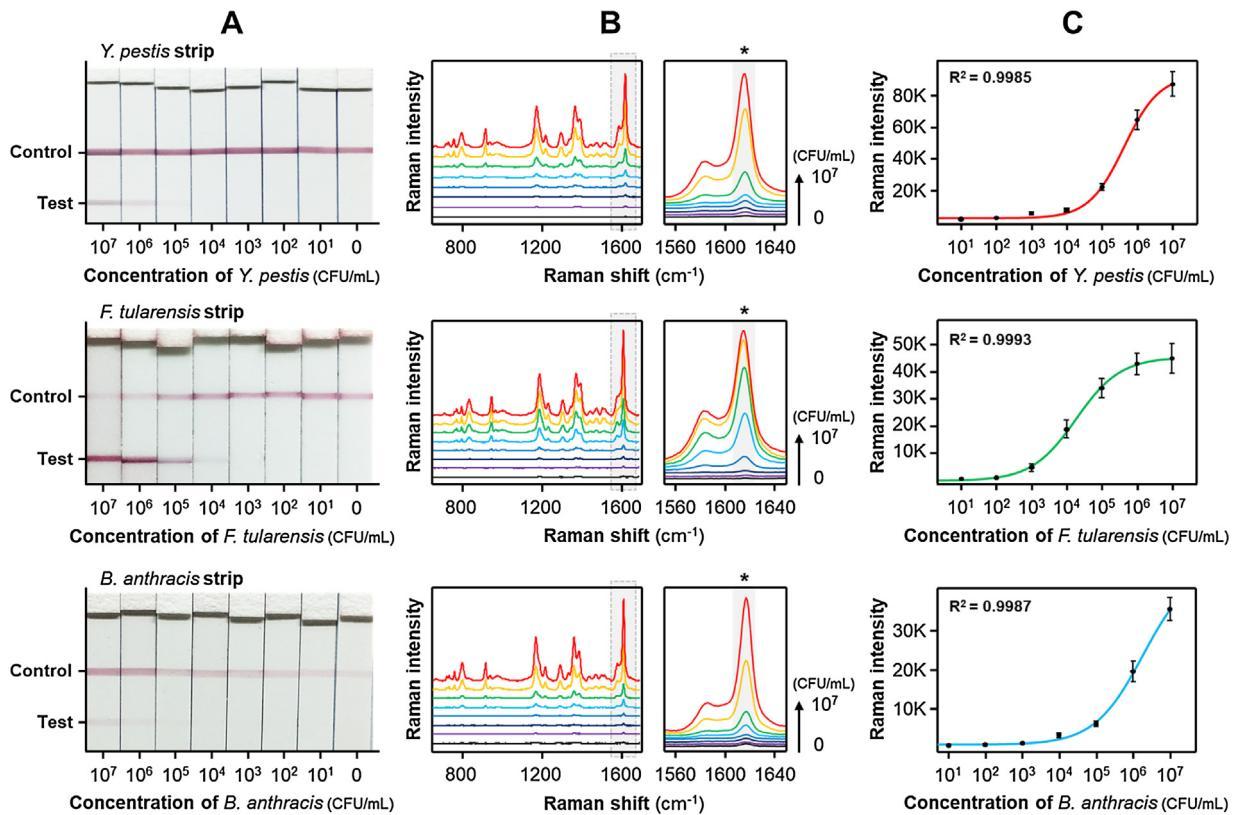
**Fig. 3.** Quantitative SERS-based assay results for three bacterial pathogens, *Y. pestis*, *F. tularensis*, and *B. anthracis*. The assays were performed in the 0– $10^7$  CFU/mL range for all three bacteria. (A) Photographic images of LFA strips (B) Raman spectra of the test line and (C) corresponding calibration curves for different concentrations (from 0 to  $10^7$  CFU/mL) of three bacterial pathogens. The error bars indicate the standard deviations calculated from five measurements.
