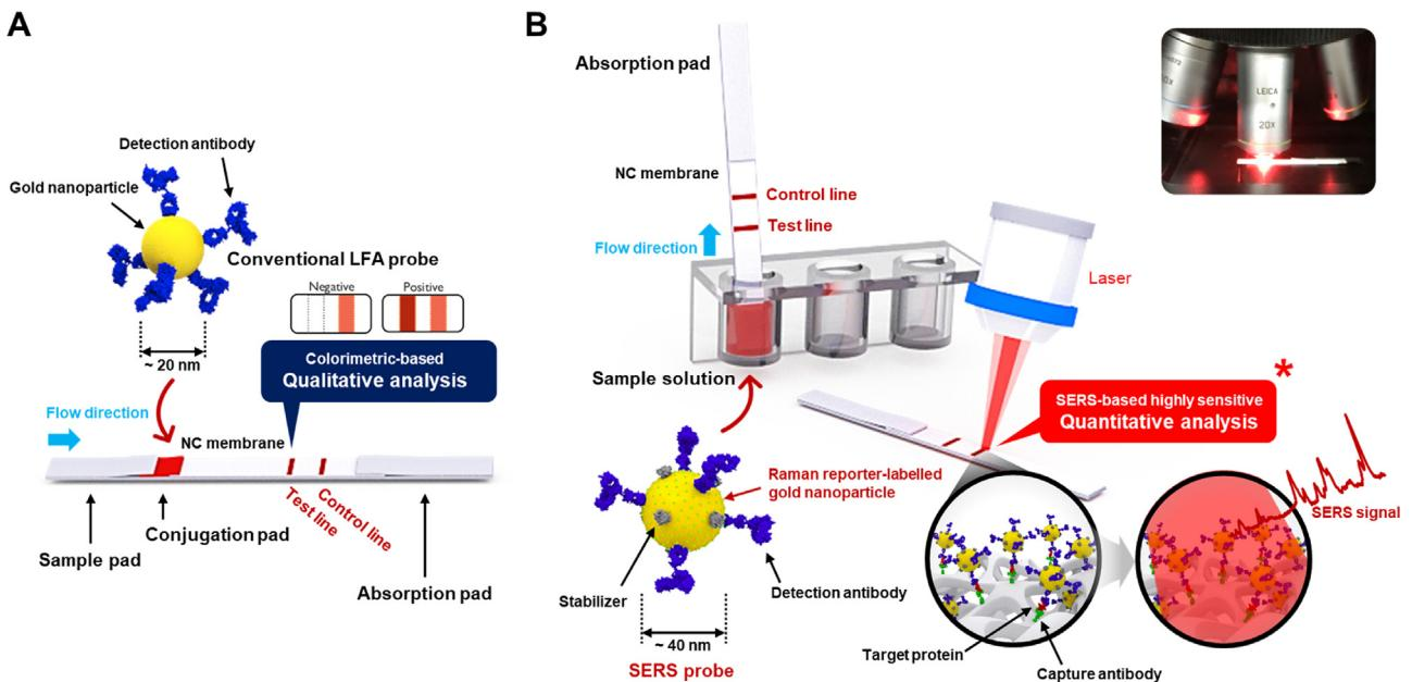
**Fig. 1.** Schematic illustration of (A) conventional LFA strip and (B) SERS-based LFA strip. In the conventional LFA strip, two color bands were observed ("on") in the presence of target whereas only one color band on the control line was observed in the absence of target ("off"). Using the SERS-based LFA strip, quantitative analysis of a specific target can be performed by monitoring the Raman intensity of a characteristic Raman peak of SERS nanotags captured in the test line.
