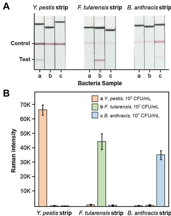
**Fig. 5.** Selectivity test of SERS-based LFA strips. (A) Digital photographic images of three strips and (B) their SERS signal intensity variations for *Y. pestis*, *F. tularensis*, and *B. anthracis*. The test concentration was  $10^7$  CFU/mL for all three bacteria. Error bars indicate the standard deviations of five measurements for each strip.
